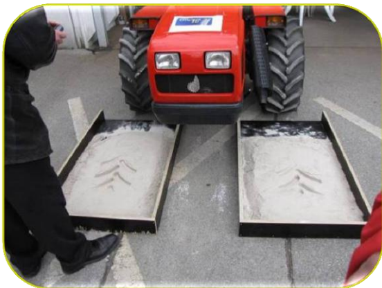
Influence of tractor tyre pressure on surface – demonstrated on sand and presented on regional Spring agricultural fair for Gorenjska region (organiser of mentioned fair - associated member Agromehanika d.d., Kranj)
