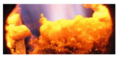
Figure 3: Slag formation in a small scale combustion system
