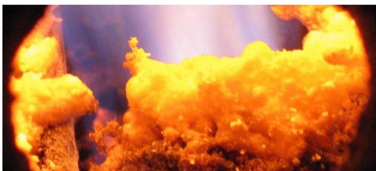
Figure 3: Slag formation in a small scale combustion system
