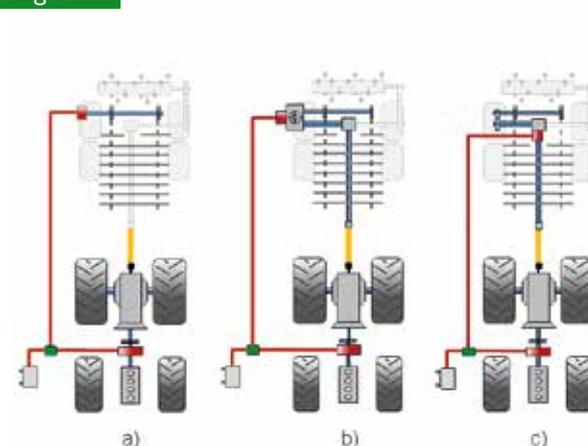
Manure spreader with chain feed drive in different agro-hybrid-structures (serial, power-split, parallel)
