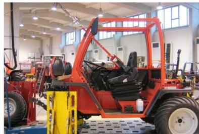
seatbelt anchorage test
