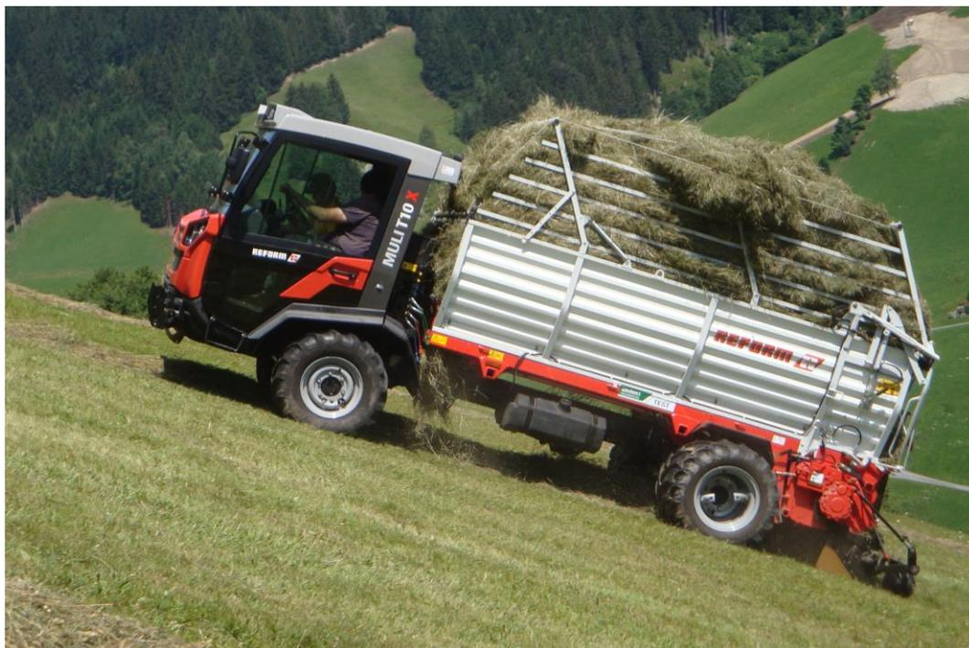
Figure 2. Transporter equipped with a loader wagon.
