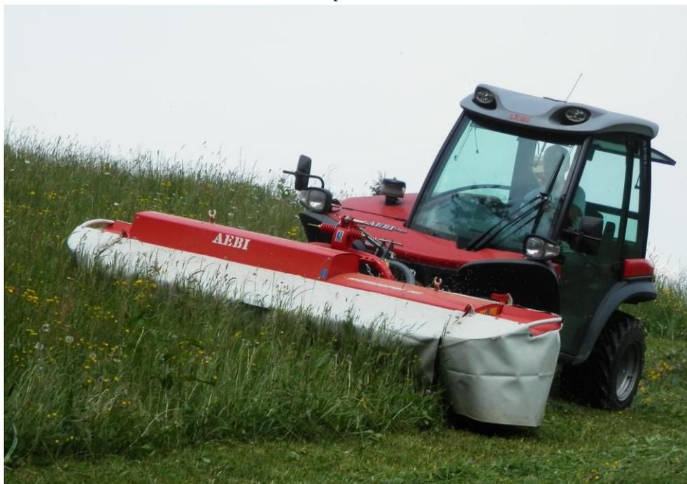
Figure 1. Two-axle mower equipped with a disk mower.
